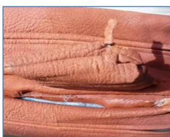
Cover Damage caused by chemicals
